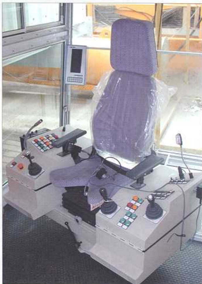
■ A Liebherr driver's seat with the EMS display mounted conveniently for the driver
