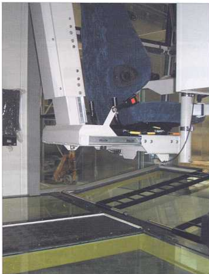
■ The Ergoseat is suspended from the cab's ceiling
